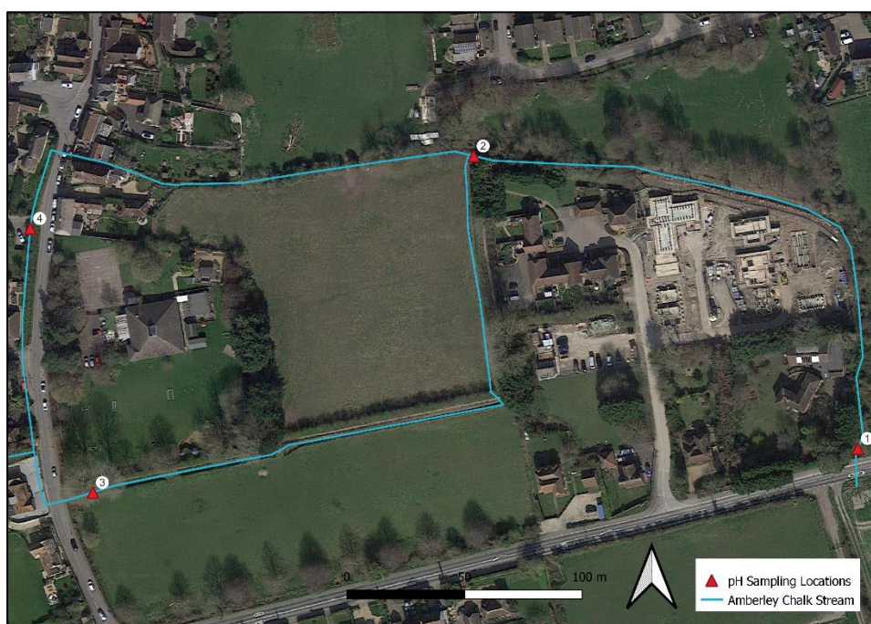
Figure 11: Map of four sampling locations used to collect data on the pH of the Amberley Stream using a digital Apera PH20 pH Tester ( \pm 0.1 accuracy; Apera Instruments, 2025).
