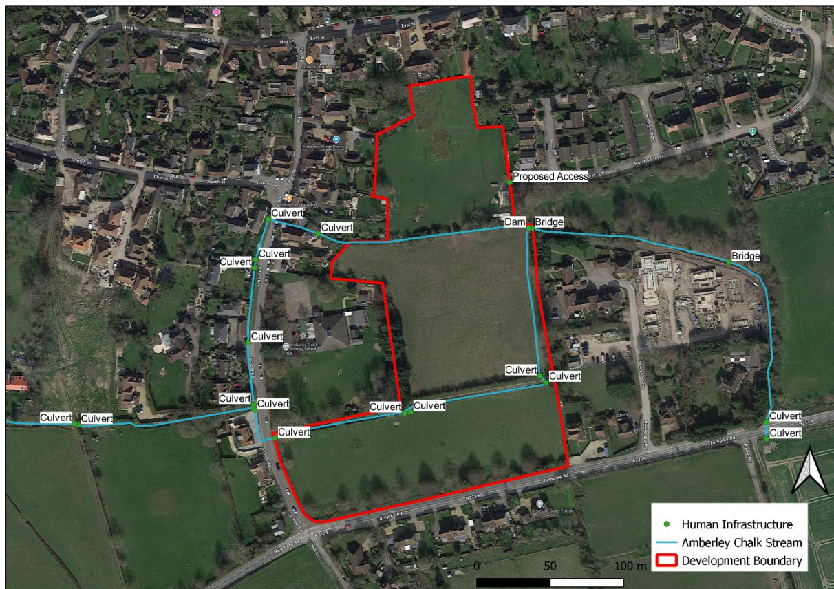
Figure 2: The route of the chalk stream in the village of Amberley, running from east to west. From its earliest identified point, the stream runs across the site of proposed development at East Street Farm, passing through multiple culverts through the village.
